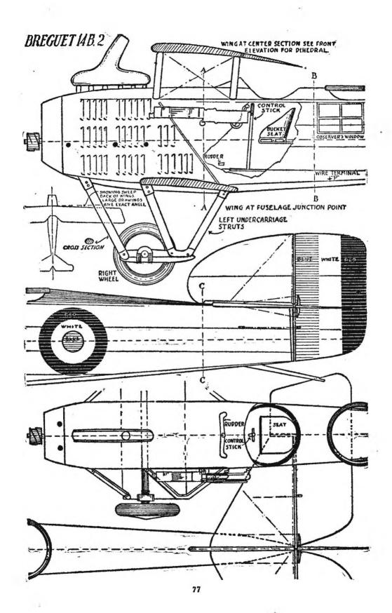
Width top wing-5 ft. 111/2 in. Bottom wing 5 ft. Gap at wing tips-5 ft. 8% in.
